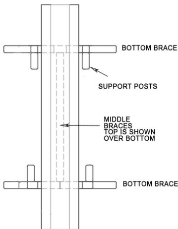
**LOG SLUICE ASSEMBLY DETAIL**
